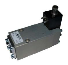
Description Function 2-2 4 ... 40 bar Operating pressure Pilot pressure 6.2 bar + 0.2 bar Nominal diameter 16 mm Valve body: Coated Materials aluminium Piston: Plastic, FDA compliant Operating temperature +5° ... +55° C Pilot valve 24V DC, 9.7W, IP 65 Net-weight 1.6 kg Pilot: V2VS2BPA Spare parts V2VS2BVB Piston & spool: V2VS2VMA Seat bush: V2VS2VSA
