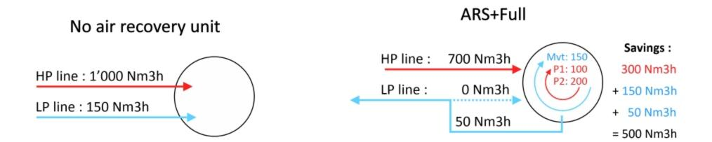
Depending on your machines, production and air network, switching OFF an HP compressor with ARS+ or a LP compressor with ARS can be considered, with significant savings on the compressor's maintenance
